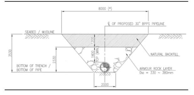
Figure 2.5 Trench Design (Type E)
