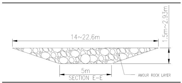
Figure 2.2 **Trench Design (Type B)**
