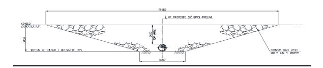
Figure 2.7 Trench Design (Type G)
