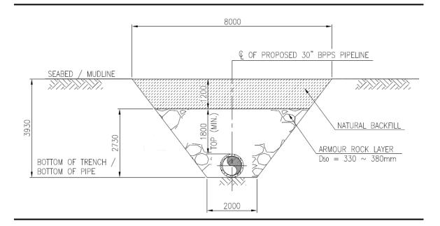
Figure 2.6 Trench Design (Type F)
