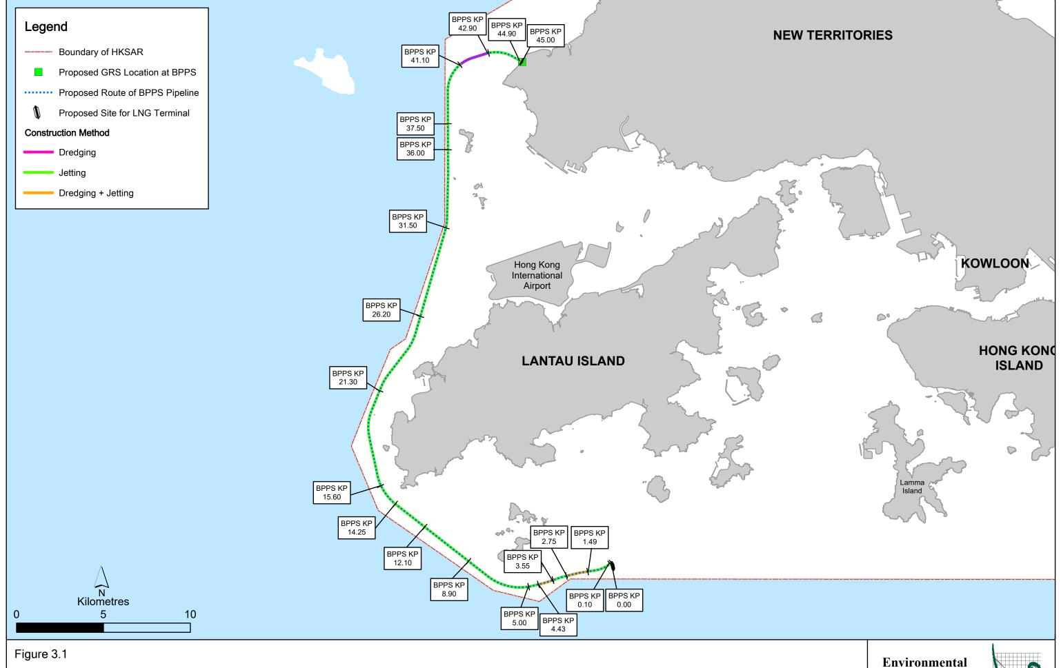
Construction Methods for the BPPS Pipeline
