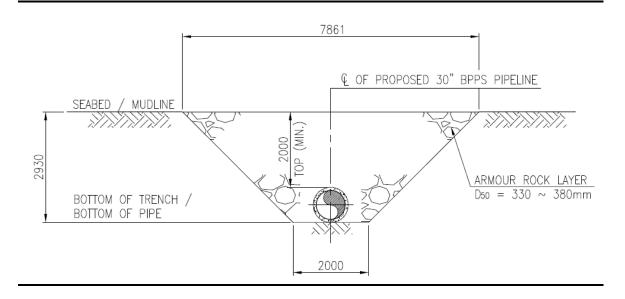
Figure 2.3 Trench Design (Type C)
